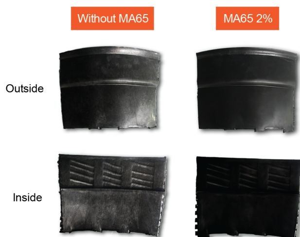
Fig 1 : Comparing silver steak of finished product with and without Elastoflex ® MA65 2%
