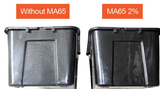
Fig 3 : Comparing silver steak of finished product with and without Elastoflex ® MA65 2%
